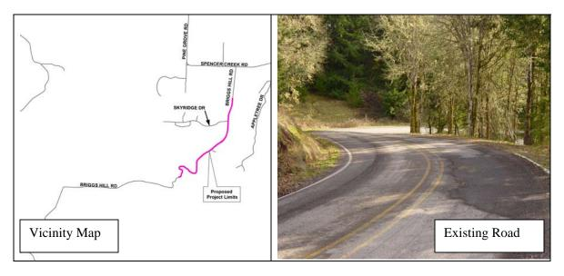
**Define the Problem:** This road segment shows up on the Lane County overlay list but was taken off due to its narrow width, inadequate base, and drainage issues.
